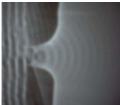
Water waves from narrow slit ripple tank.
